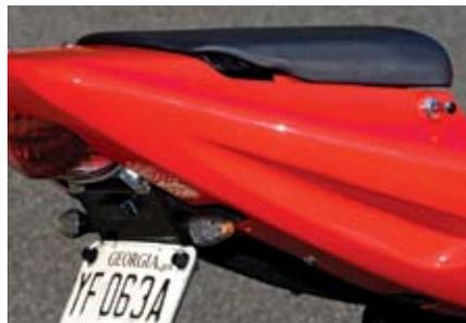
The rear grab rail was deleted, subtracting another 2.2 lbs. This left two unsightly indents under the passenger seat, but we intend to replace it with a slick-looking solo seat cowl anyway.
