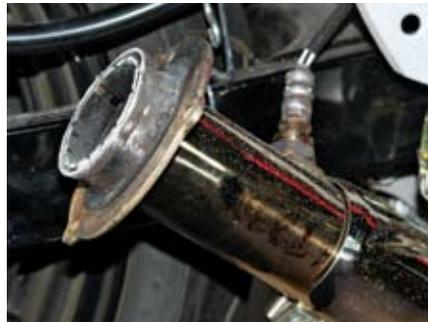
The toughest part about bolting on the Two Brothers exhaust was hacksawing this flange off the mid-pipe. The new muffler is sure to increase performance—and it lopped off 74 pounds.
